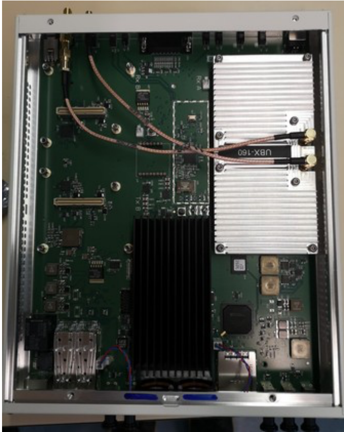
Fig. 4. ETTUS X310 with installed UBX-160 daughterboard on slot A and internal cables leading to the ports labeled B.
